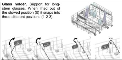
2-position fold-down supports (1-2). In position 1 (vertical) they can be used to take plates, while in position 2 (slanted) they provide support for long-stem glasses which will be held in place by the **glass holder**. Adjustment: raise point **P** as shown until the support turns into position 2.
