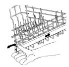
Version B: with adjustment in three positions on both sides.
