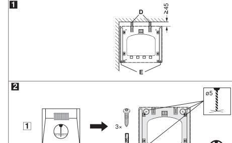
Fold out spacers D in order to keep distance to the back wall.
