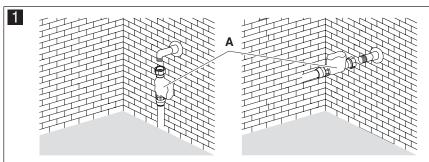
Preferred alignment for Aquastop valve block **A** (sound-optimized installation):
