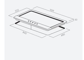
AGH91X Series Hob Specifications Total Gas Consumption: 32.4 mj/H Electrical Connection: 10AMP GPO
