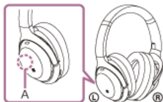
A: Location of the built-in antenna
